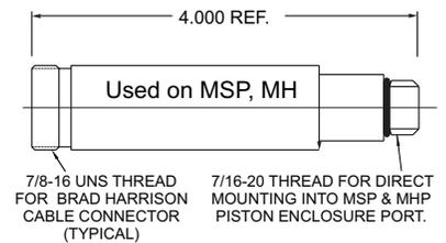
**TRABON® FS<sub>MECH</sub> - TYPE PROXIMITY SWITCHES - 3 PIN, 4 PIN, 5 PIN, EXPL. PROOF**
